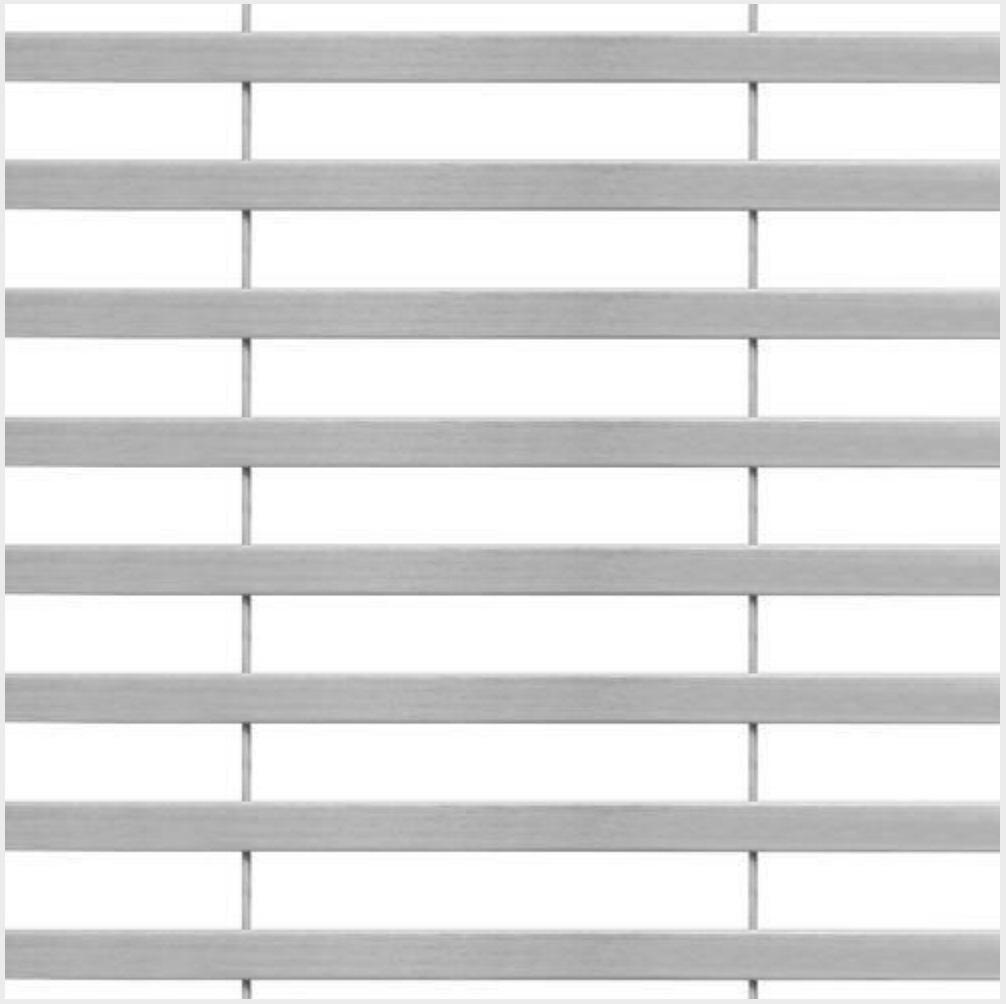
ARRAS D08160 Open area: 66,6 % Weight: 6,8 kg/m² Slot: 16 mm Material: PZ System: H P
