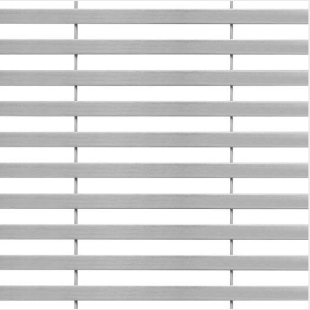
ARRAS D08100 Open area: 54 % Weight: 8,6 kg/m² Slot: 10 mm Material: PZ System: H P
